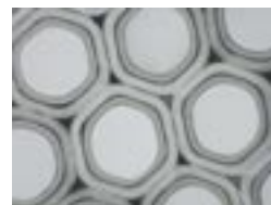
(Left) Incom ultrathick absorbing microcapillary plate.
